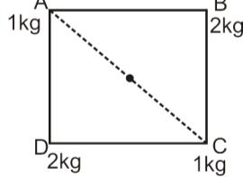
Since masses at A and C are same, masses at B and D must be same to get centre of mass exactly at geometric centre.
